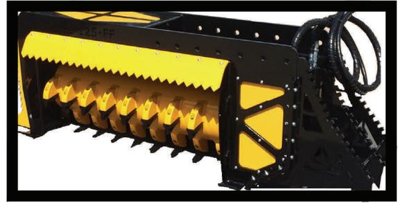
A hydraulic motor is matched to the hydraulic output of your Machine for superior power delivery. The direct drive coupling eliminates high maintenance belts and pulleys. This ensures you get the maximum performance from your mulcher using your standard hydraulic system. The Machines are fitted with two main high pressure hoses for hydraulic inlet and outlet, and in most cases, don't require a case drain.
