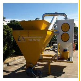
The unit can deliver a metered discharge rate as required and can be either belt or screw driven dependent upon product. Discharge rate is controlled via a programmable interface.
