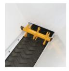
Due to the larger hopper the Bag-it 30 has the addition of an anti bridging device fitted above the feed belt, designed to free up moist or lumpy material making for a smooth and consistent fill.
