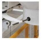
A simple bag clamping device operates as soon as the pedal is engaged. Sitting on both sides of the chute the clamps make sure that the bag stays in place when the product enters the bag, releasing when the bag is full.
