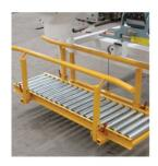
Included is a fully height adjustable transverse roller ramp, mounted under the chute and capable of filling bags from 10 to 100 litres in standard form.
